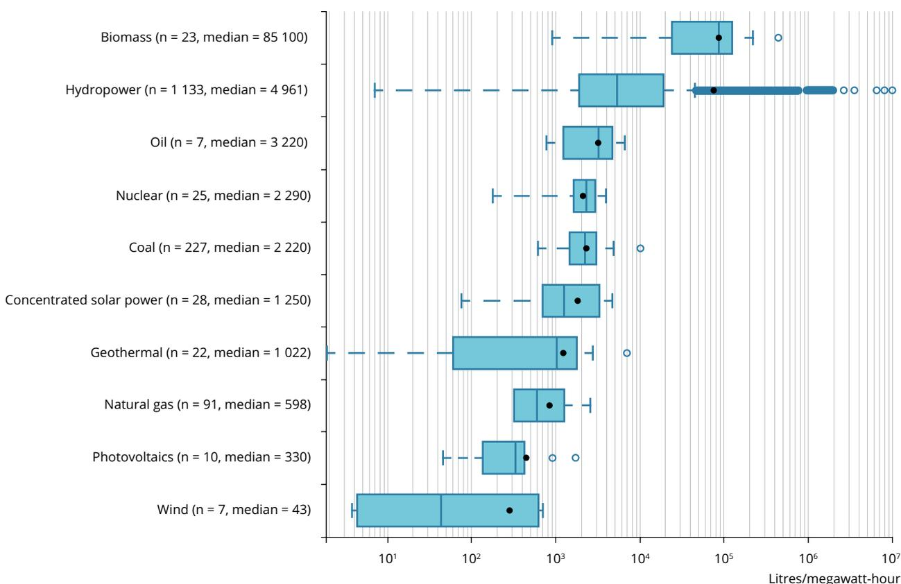
**Notes:** Water consumption is shown on a log scale. Circles represent the outliers, while the dots represent the average for each power type. CSP, concentrated solar power; mdn, median value of water consumed; PV, (solar) photovoltaic.
