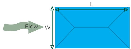
If rectangular houses cannot be oriented along the flow as shown, keep L less than double side W
