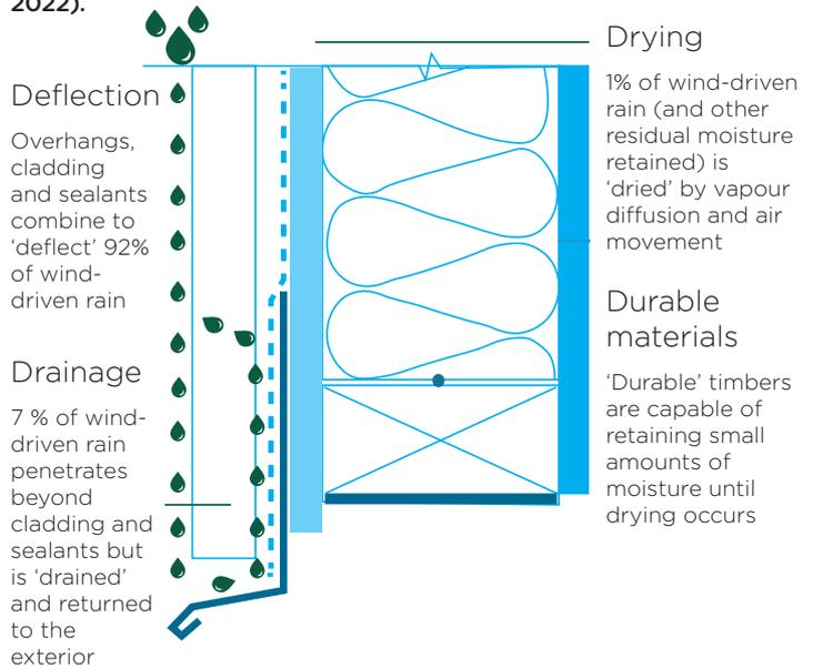
Rainscreen cladding is a form of double-wall construction that uses an outer layer to keep out the rain and an inner layer to provide thermal insulation, prevent excessive air leakage and carry wind loading (Proteus Facades, n.d.). Section 3 provides further information on solutions for heavy precipitation.
