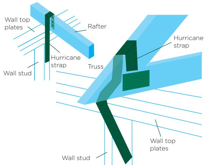
Under the roof, the linkage between the roof and the walls should be reinforced to prevent uplift. For instance, **hurricane straps and clips** (Figure 19) help fasten the roof to the walls of a building in case of high winds.
