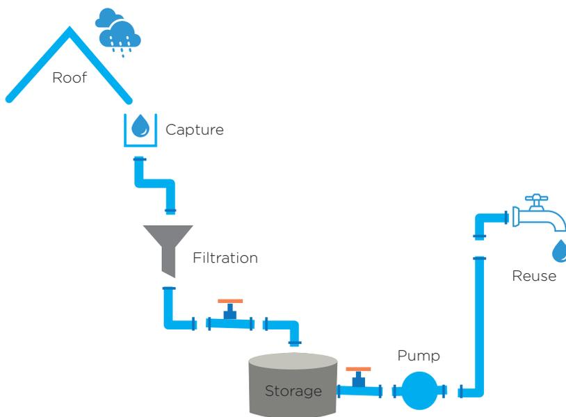
**Downspouts** can also be connected to water storage solutions such as rainwater tanks to provide grey water for toilets or watering plants during dry periods (Figure 31). Water collected in this manner is not suitable for drinking unless it is further filtered and exposed to ultraviolet treatment (Kirton, n.d.).
