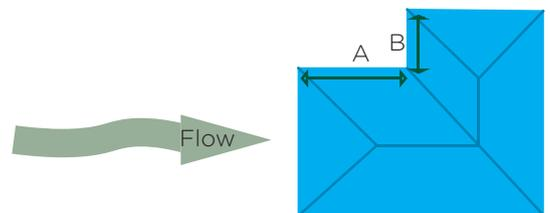
If the longer leg of L-shaped houses cannot be oriented along the flow as shown, keep side A less than 1.5 times side B
