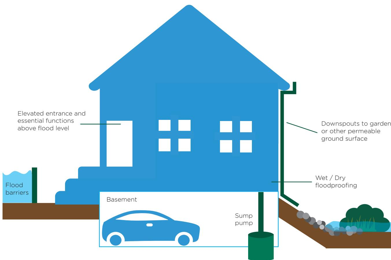
These solutions will be appropriate for different levels and duration of flooding. For short-term floods, and with a low flood level (up to 0.3 metres), an early warning system in combination with temporary shields of openings to buildings and moving essential functions up in the building might be sufficient. In regions that are prone to floods of long duration, or high flood levels, more drastic solutions will be required, such as adequate foundations and the use of water-resistant materials.
