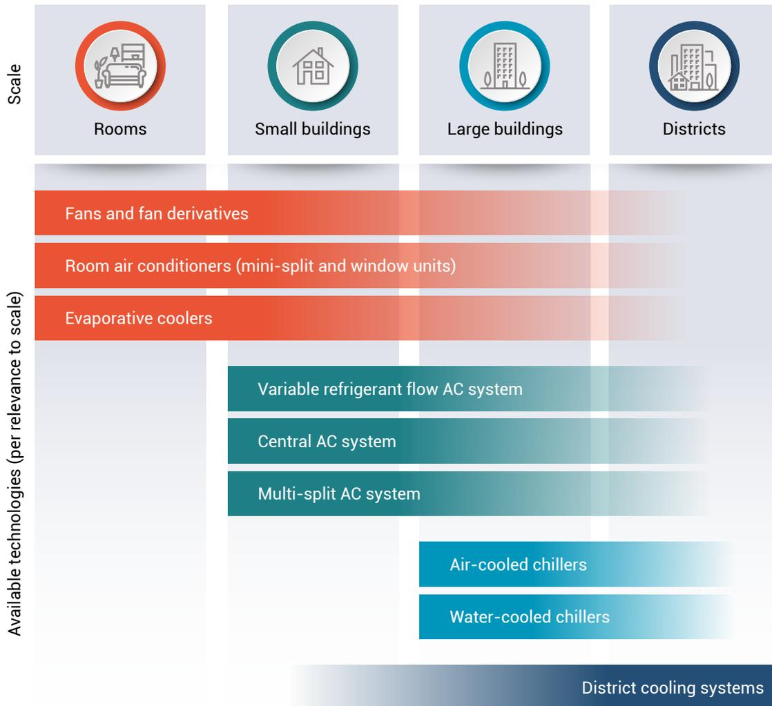
Note: Shading represents each cooling equipment's applicability at the corresponding building scale.
