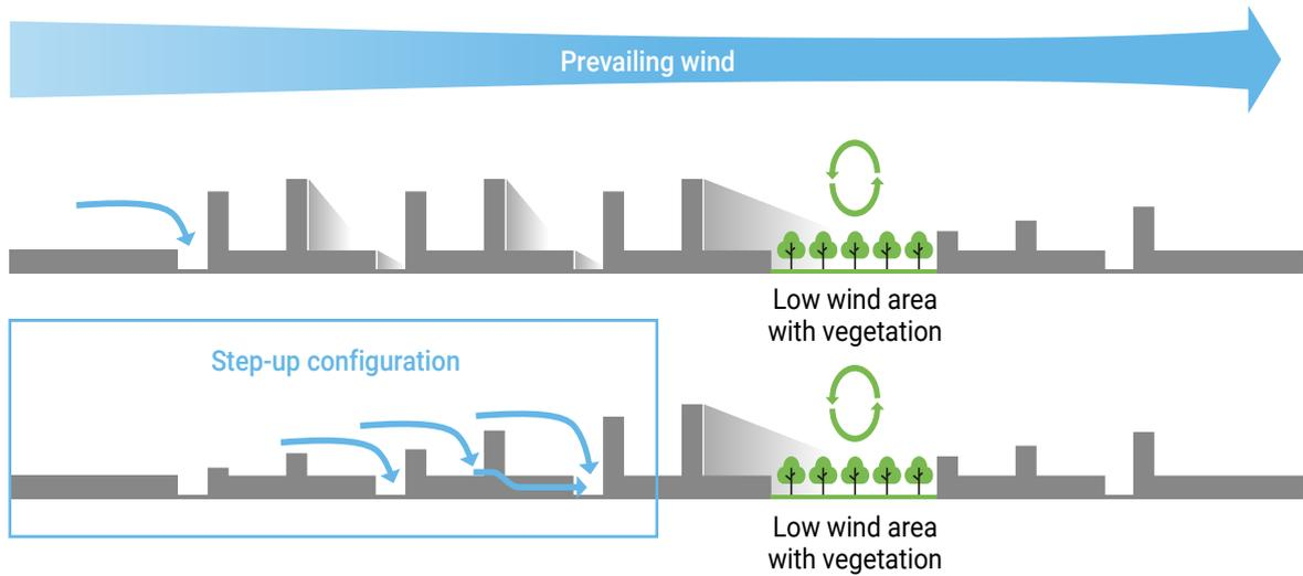
Note: In the figure, taller buildings of relatively uniform height produce wind shadows and reduce ventilation in urban canyons (top). A step-up configuration, in which downwind buildings become progressively taller, increases pedestrian-level ventilation (bottom). Where wind shadows are unavoidable, green spaces provide cooling convection.
